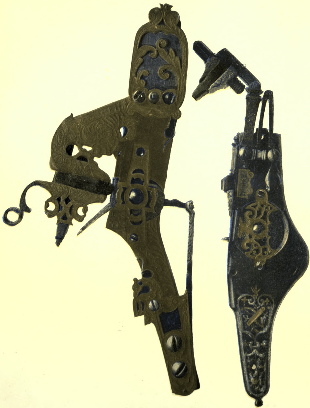
PLATE VIII.—Wheel-lock of bright steel, with engraved and pierced brass. German, 17th Century.
